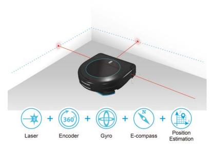
LEGEE is the abbreviation of the unique navigation system that integrates Laser, Encoder, Gyro, E-compass and Position Estimation together to detect and measure the surroundings. LEGEE detours around the furniture and other objects while precisely plans the cleaning path to clean the entire floor of your home.
